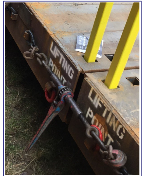
Chain ratchet close-coupling system
